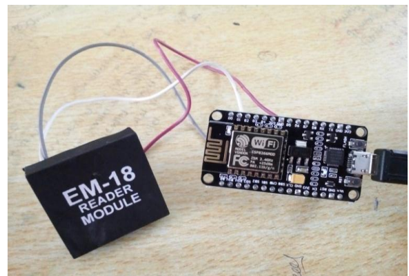
Fig 4 Connection Between RFID and ESP wifi Controller:
